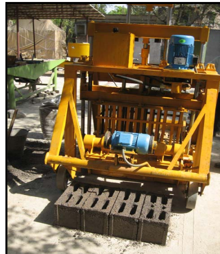
Production of hollow walling blocks
