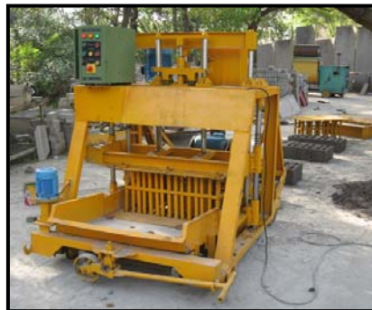
Production platform for TARA GreenCast Panels
