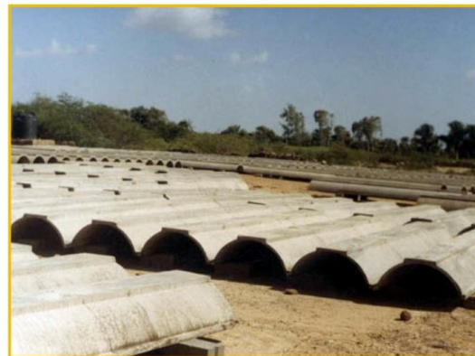
Finished Ferrocement roofing channels
